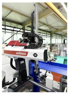
The new WX90 sprue removal systems with rotary servo axes are equipped with an R9 control system and thus completely integrated in the production cell.
